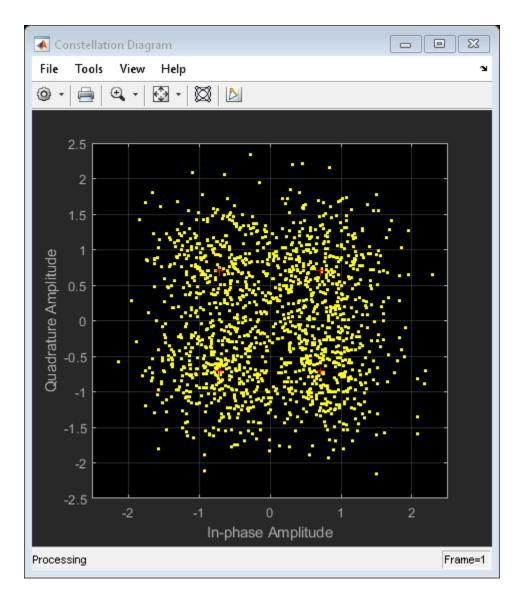
Demodulate the noisy symbols to obtain soft bits, convolutionally decode the soft bits, and display the number of erroneous bits.
