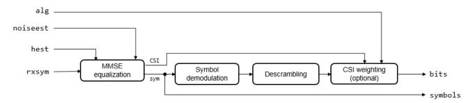
If the resource element grid across all possible EPDCCH antenna ports is input, the function extracts all EPDCCH resource elements and performs EPDCCH decoding for all possible EPDCCH candidate locations. The function assumes the input symbols were already equalized. Each EPDCCH candidate is descrambled individually during EPDCCH search.
