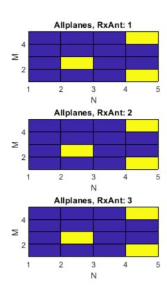
Create a 4D channel estimate grid to extract resource elements. Extract resource elements from the channel estimate grid. Show the locations of these extracted resource elements. Addressed resource element locations contain 1.
